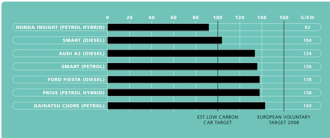
The Honda Insight achieves 92 g/km well-to-wheel CO<sub>2</sub> emissions, which demonstrates that there are already hybrid technologies on the market that would be classified as ‘low carbon’. Other options that EST expects could potentially contribute towards a 2010 low carbon car target include future:
